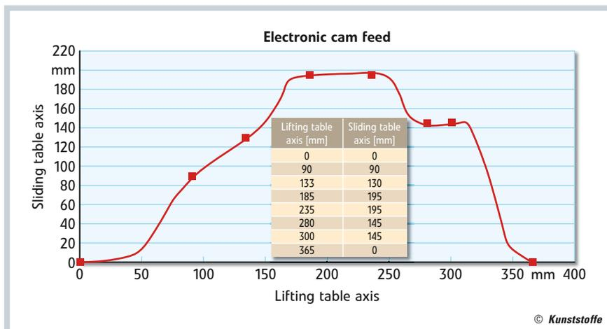
**Fig. 4. A lifting table/sliding table control following the master-slave principle permits precise coupling of the movement sequences**
