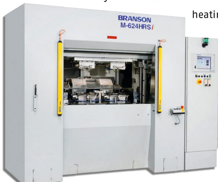
**Fig. 1.** The M-624HRSi all-electric vibration welding unit with infrared pre-heating (CVT) was presented at K2007
